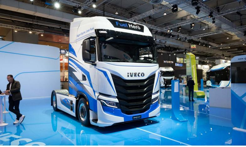
Above: The S-Way Fuel Hero features a new Cursor 13 365 kW (490 hp) engine and it is offered with a specific configuration of options which can improve overall fuel efficiency by up to 4%. Iveco's Professional Fuel Advising Service can deliver a further 4% in savings.
